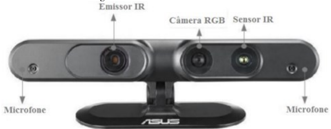
Figura 3.13 – Sensor Xtion PRO LIVE .
