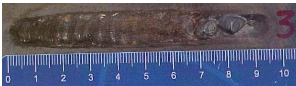
(c) Gás de proteção 15,0 l/min; gás de arraste 1,0 l/min; gás de plasma 2,0 l/min
