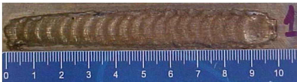
(a) Gás de proteção 15,0 l/min; gás de arraste 2,0 l/min; gás de plasma 2,0 l/min.
