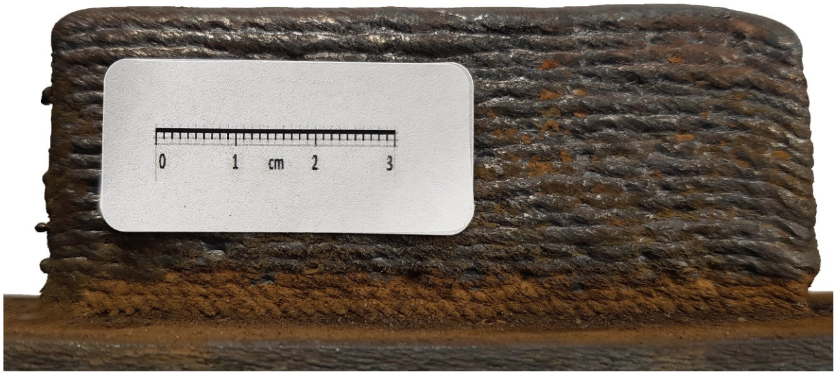
Figure 27: Sample 1, side view. CMT variant, as welded.
