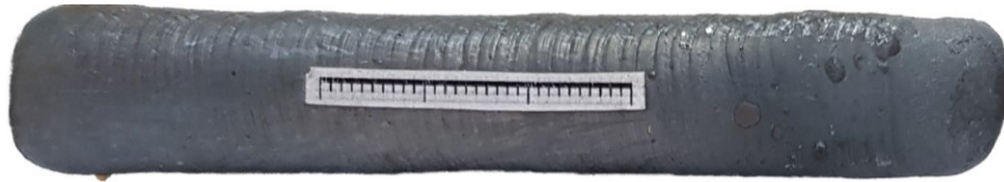
Figure 30: Wall top view. CMT.
