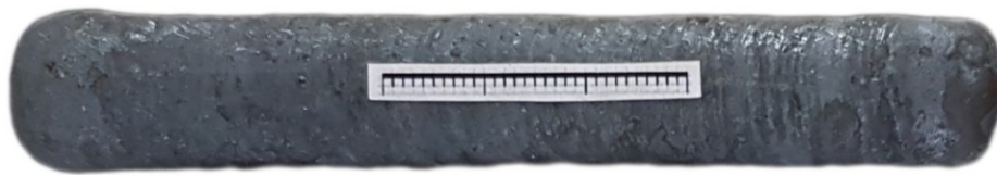
Figure 31: Wall top view. CMT Pulse.
