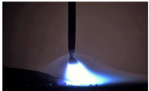
Figure 6: Positive Polarity. The arc anchors at the end of the droplet. [11]
