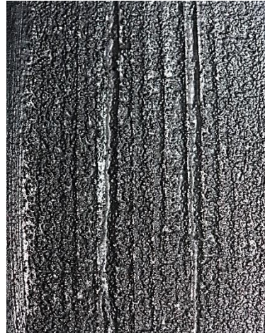
Figure 38: Scratched surface pattern of same specimen of figure 37 with 2x zoom.
