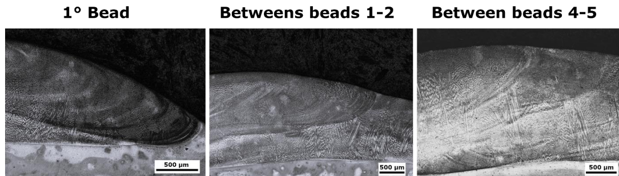
Figure 4. Optical-microscope panoramic of the inter-bead region of the process CWF-GTAW.
