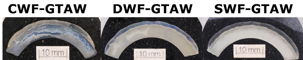
Figure 3. Comparative macrographs of the coatings applied by the CWG-GTAW, DWF-GTAW and SWF-GTAW processes.
