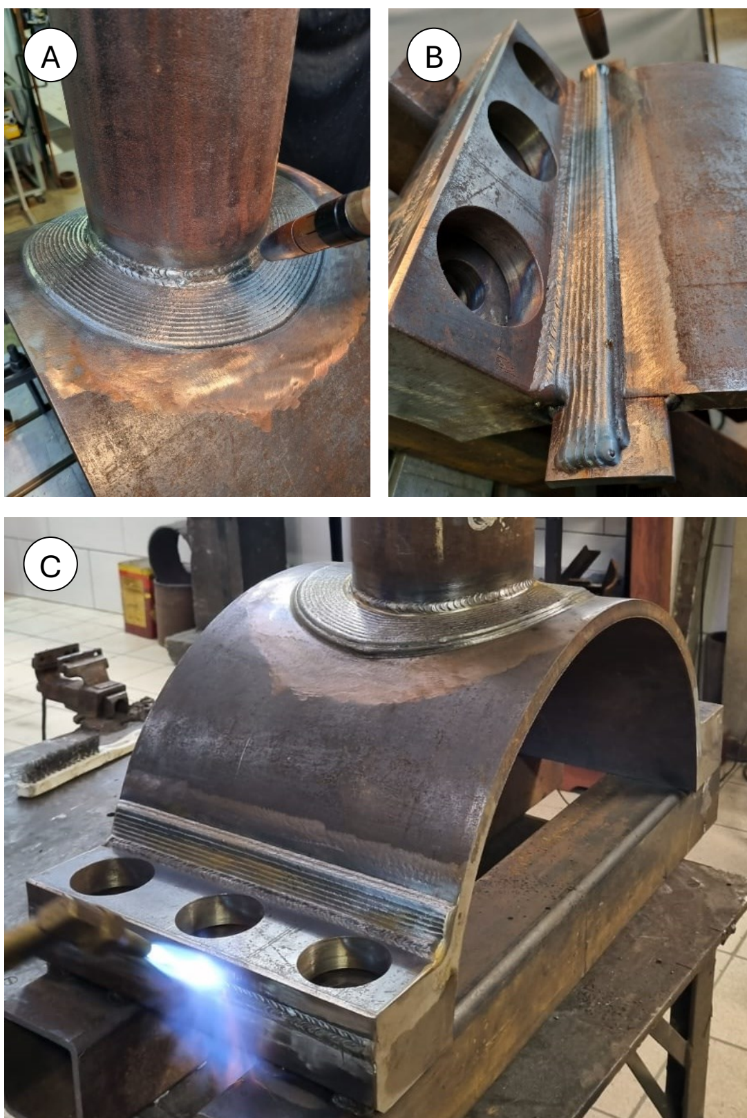
Figure 5 - Result of the additive manufacturing reinforcement process on a clamp for oil and gas pipeline repair.
