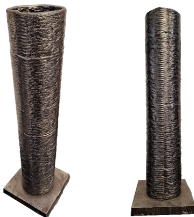
Figure 7. Surface appearance of the printed cylinder using the temperature control system.
