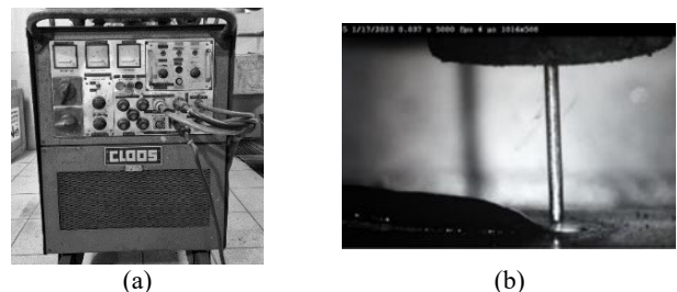
Fig. 1 In (a) CLOOS power source; (B) Buried arc condition (Silva, R. et al., 2023). Video available at: https://youtu.be/3kJIvAdYBY
