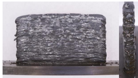
Figure 18 – Wall made with AM by ECP 1, front and side.
