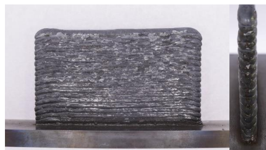
Figure 20 – Wall made with AM by RWF 3, front and side.
