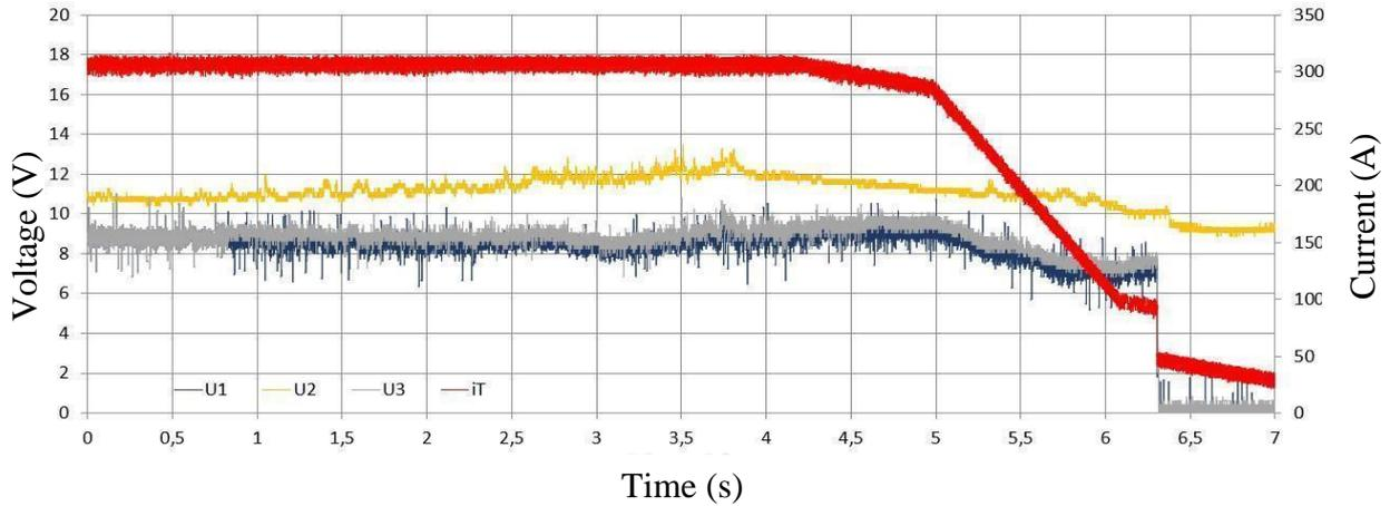
Figure 7 - Multicathode TIG with 3 electrodes and wire feed speed of 3 m/min
