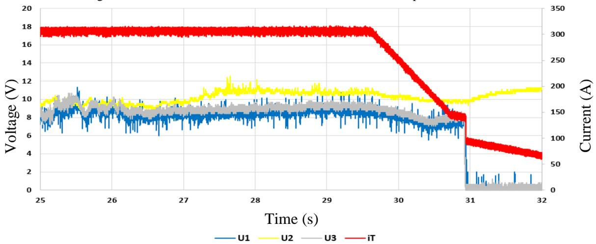
Figure 8 - Multicathode TIG with 3 electrodes and wire feed speed of 4 m/min
