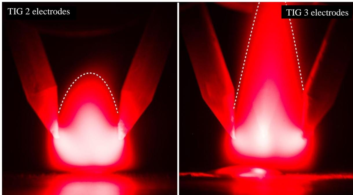
Figure 5 - Multicathode TIG arcs for the 2 and 3 electrodes process
