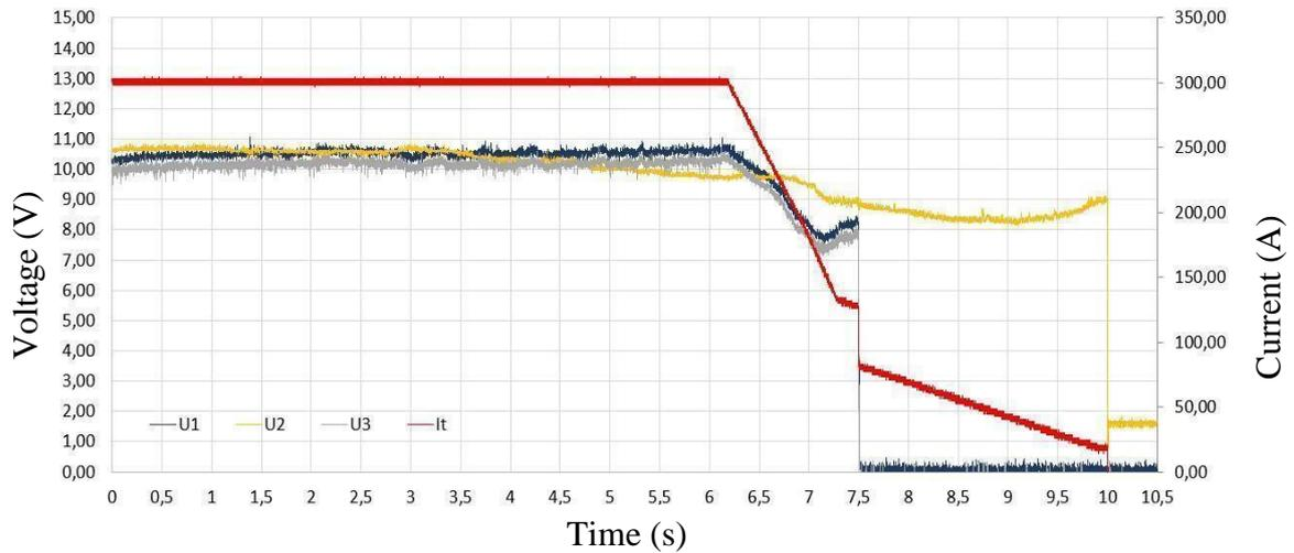
Figure 4 - Triple electrode TIG: current (red) and voltages (gray, yellow and blue)
