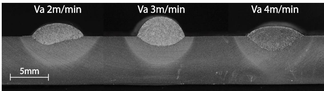
Figure 10 - Macrographs of the multicathode TIG with wire feed. Va: Wire feed speed
