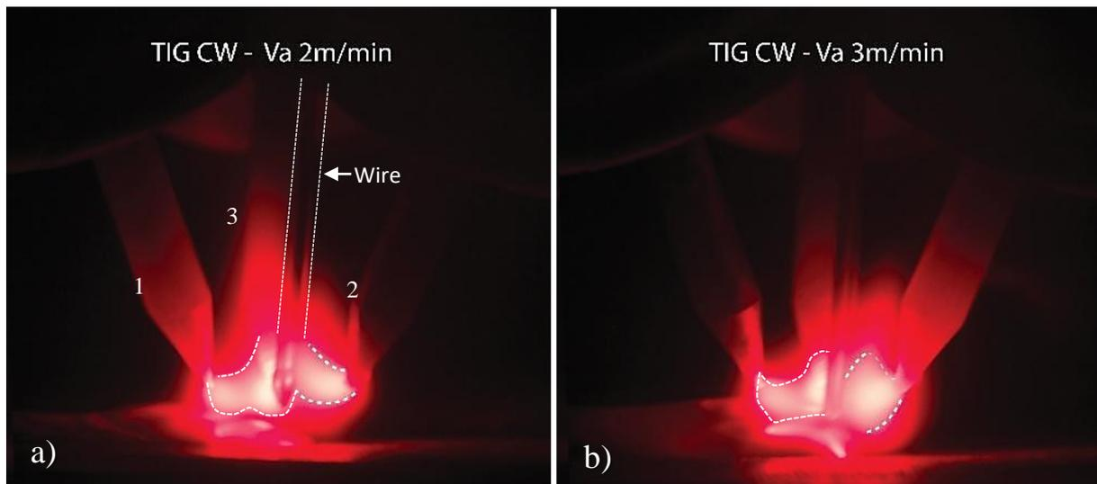
Figure 9 - Interactions of arcs with cold wire (CW) feed: a) intermittent transfer b) bridge transfer. Va: Wire feed speed
