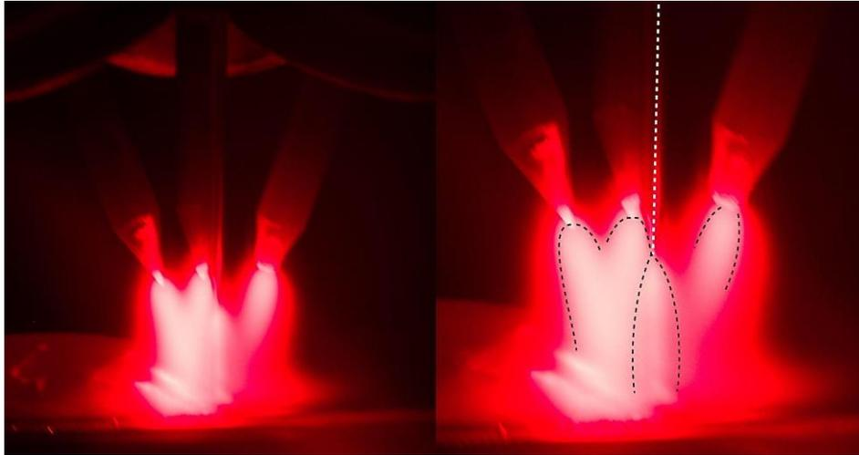
Figure 12 - Morphology of the simultaneous arcs in the TIG-MIG Multicathode Hybrid process
