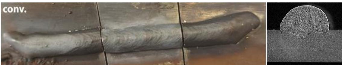
Figure 13 - Multicathode TIG-MIG process weld bead
