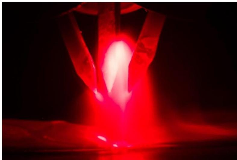
Figure 11 - Demonstration of the feasibility of operating the TIG-MIG process
