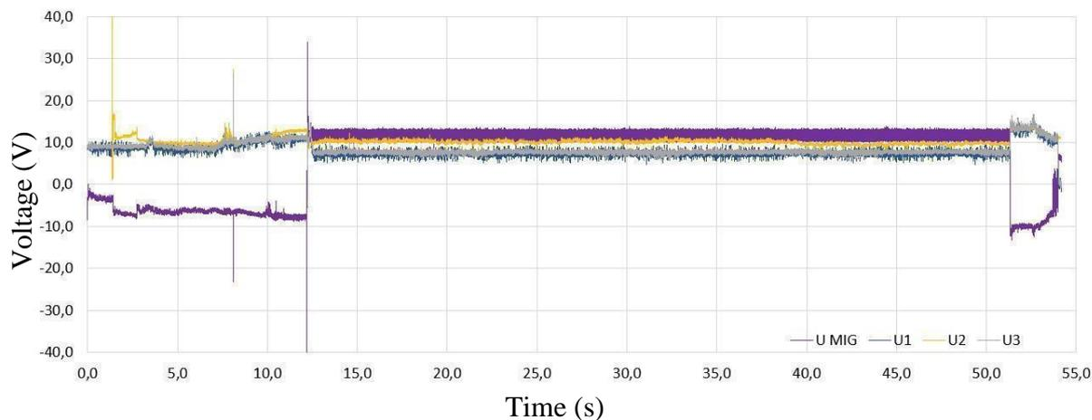
Figure 14 - Voltage signals of the hybrid TIG- MIG Multicathode process
