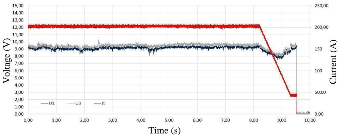
Figure 3 - Double electrode TIG: current (red) and voltages (gray and blue)
