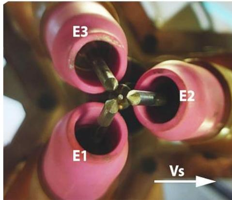
Figure 2 - Arrangement of the electrodes according to the displacement of the torch ( $V_s$ )
