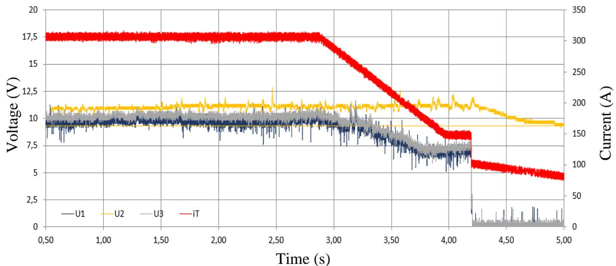
Figure 6 - Multicathode TIG with 3 electrodes and wire feed speed of 2 m/min
