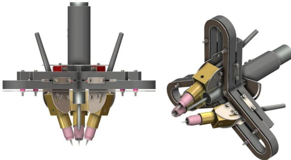
Figure 1 - CAD environment model of the TIG-MC torch
