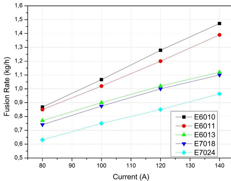
Figure 5. Melting rate for the different 3.25 mm electrode specifications.
