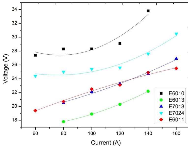
Figure 2. Static characteristic of the arc in SMA welding.
