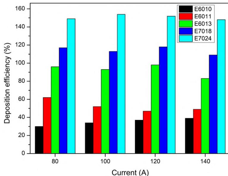
Figure 7. Deposition efficiency for the different 3.25 mm electrode specifications.
