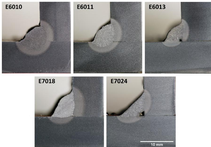
Figure 3. Macrographs of the welds with 120 A.
