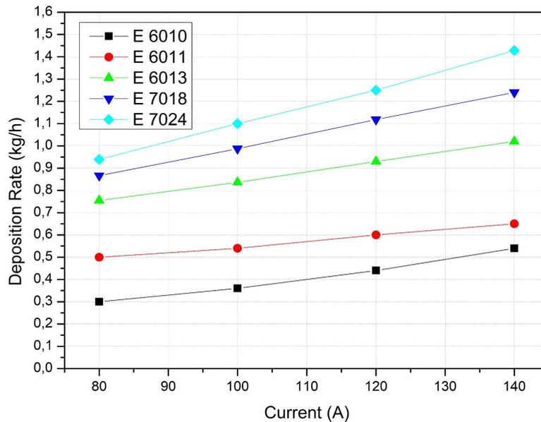
Figure 6. Deposition rate for the different 3.25 mm electrode specifications.
