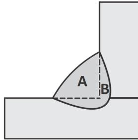
Figure 1. Geometric representation of the added area (A) and penetrated area (B) of a weld bead.
