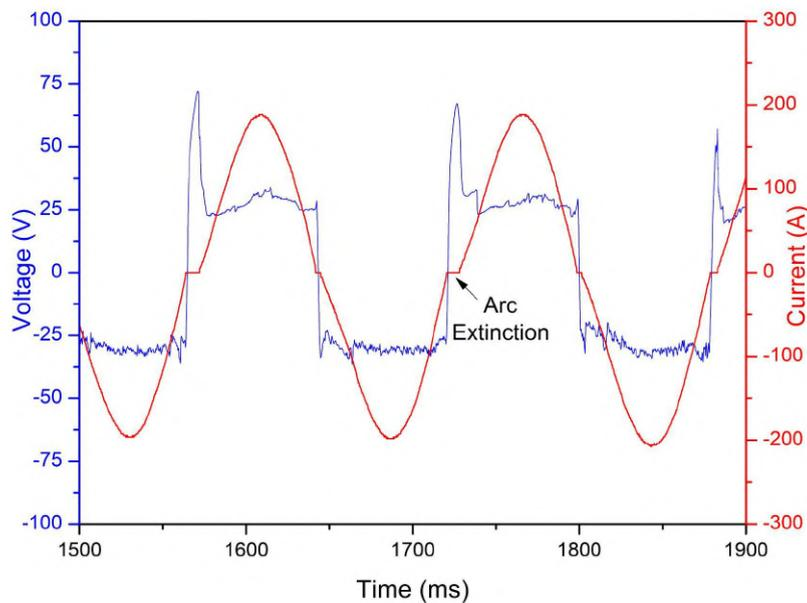
Figure 10. Voltage and current signals obtained in AC welding with E6010.
