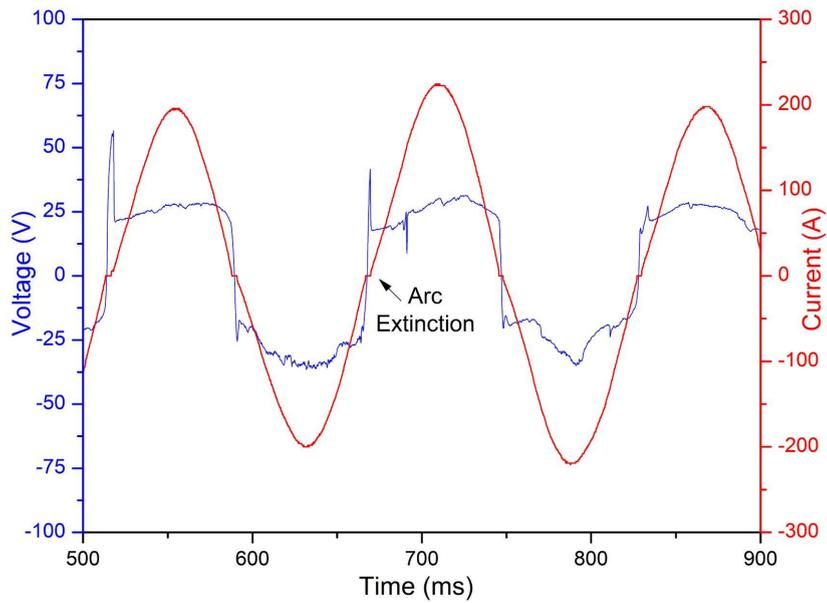
Figure 9. Voltage and current signals obtained in AC welding with E7018.
