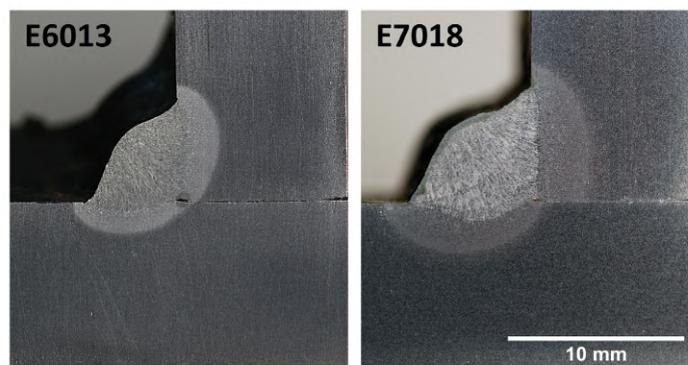
Figure 4. Macrographs of the welds with 140 A.
