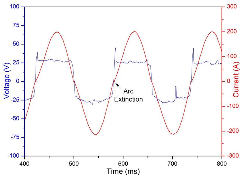
Figure 8. Voltage and current signals obtained in AC welding with E6013.
