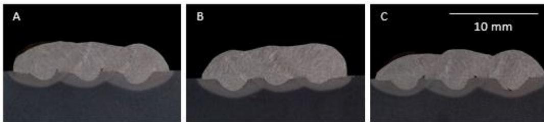
Figure 11 - Experiments for three overlap weld beads. A - Nominal center calculated distance; B - Nominal center distance less 10%; C - Nominal center distance plus 10%.
