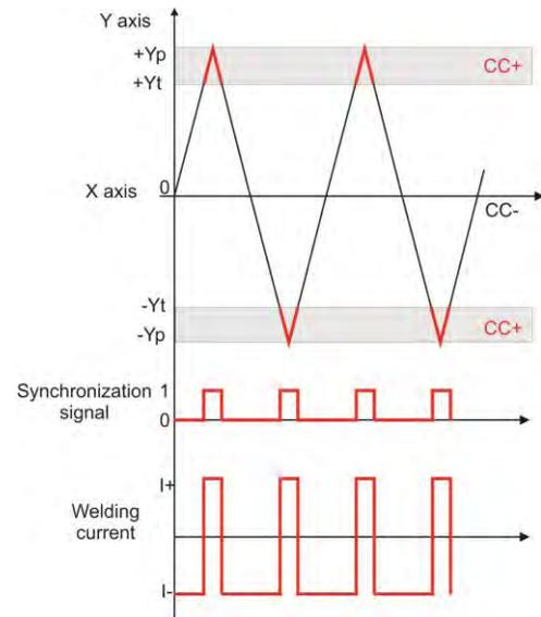
Figure 5. Synchronization logic of MIG/MAG O-PS.
