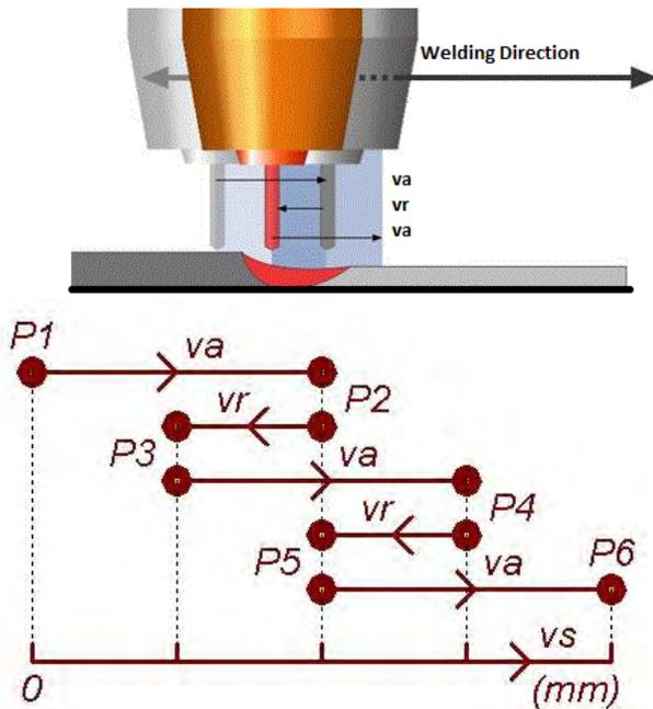
Figure 10. Switch-back oscillation technique:  $v_a$ : forwards movement;  $v_r$ : backwards movement
