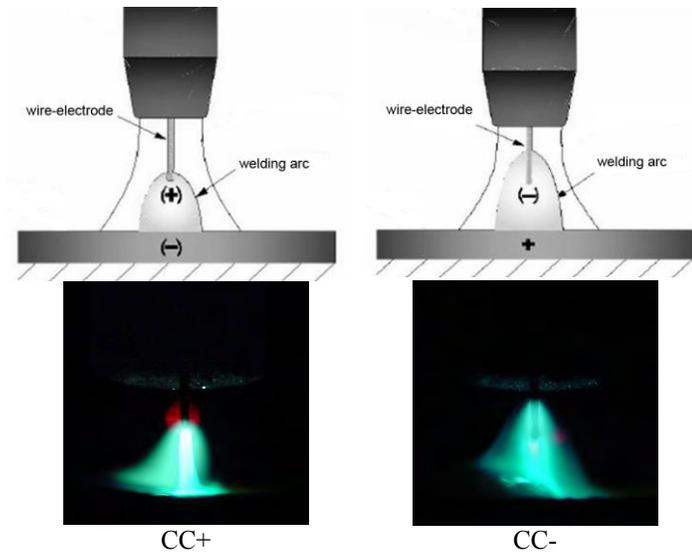
Figure 1. Arc-wire coupling for indirect polarity (CC+) and direct polarity (CC-) MIG/MAG welding (adapted from Cirino, 2009).
