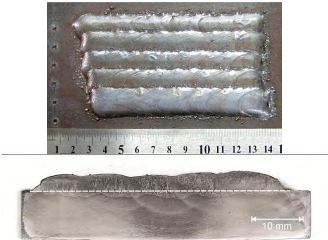
Figure 8. MIG/MAG O-PS produced weld coating.
