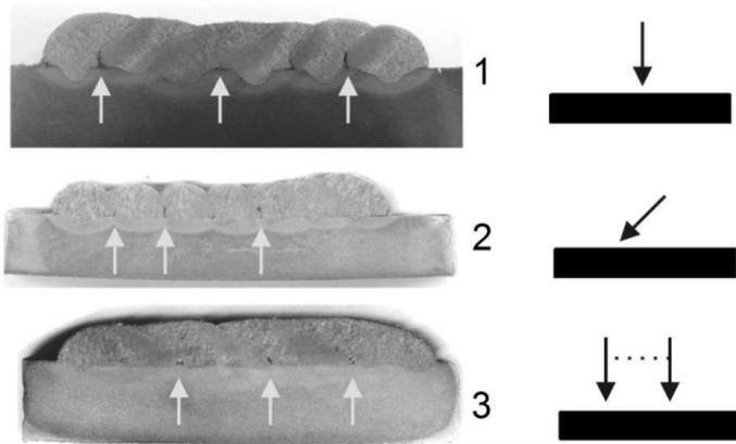
Figure 3. Coating layer deposited with MIG/MAG CC-.
