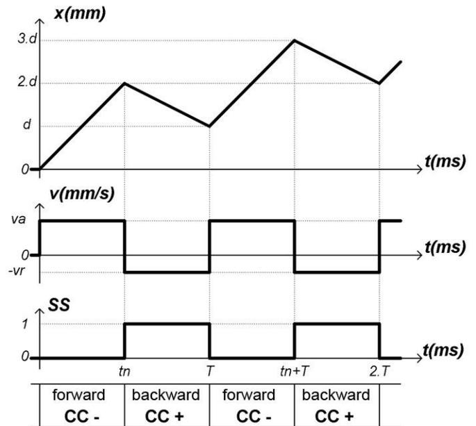
Figure 11. MIG/MAG O-PS switch-back oscillation technique.
