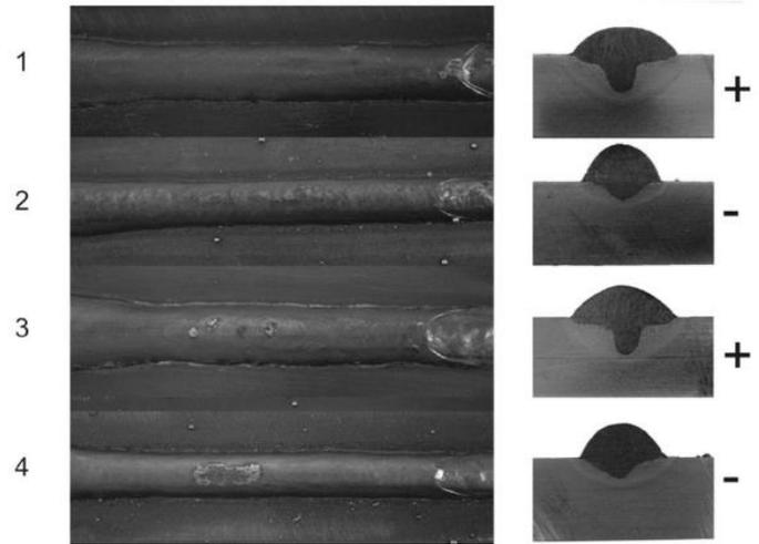
Figure 2. Effects of negative polarity MIG/MAG welding over weld seam geometrical profile (Schwedersky, 2007).
