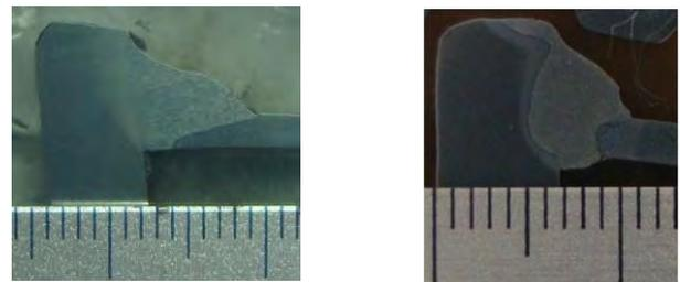
Figure 12. Left: Switch-back MIG/MAG O-PS produced weld; right: constant polarity (CC+) switch-back MIG/MAG. (scale in mm).
