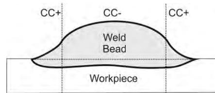
Figure 4. Appropriate bead geometry for weld coating and functioning of the oscillation-polarity synchronization.
