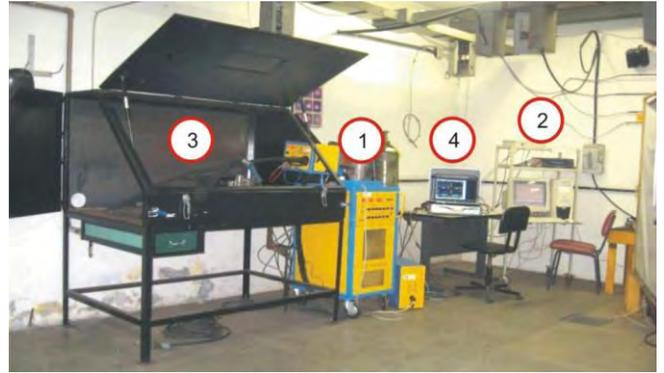
Figure 7. Welding tests rig: 1: power source; 2: CPU running SAC; 3: manipulator; 4: portable data monitoring system.
