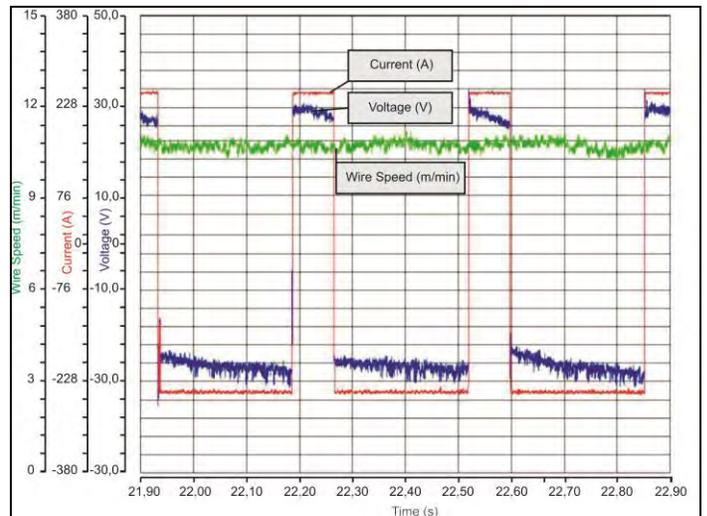
Figure 9. Oscillograms of MIG/MAG O-PS coating welding parameters.
