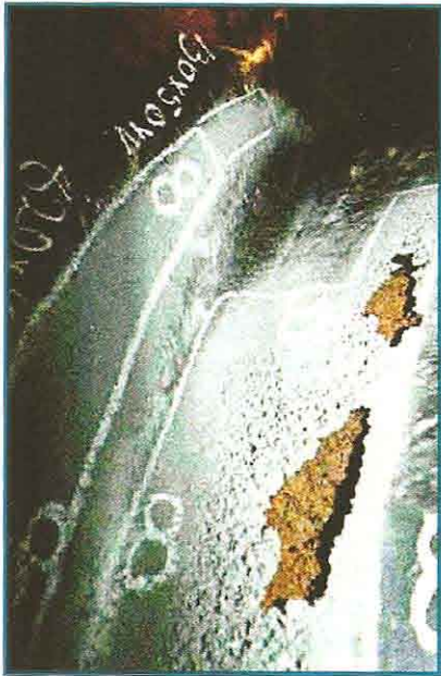
Fig. 2. Cavitation-eroded area in detail.
