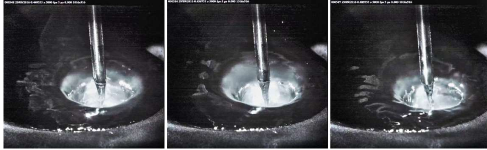
Figure 6 – Crater formed in the DynaFlex-Arc GMAW (high speed video on LABSOLDA's Channel on - https://youtu.be/RkpVX2cv1qc ).
