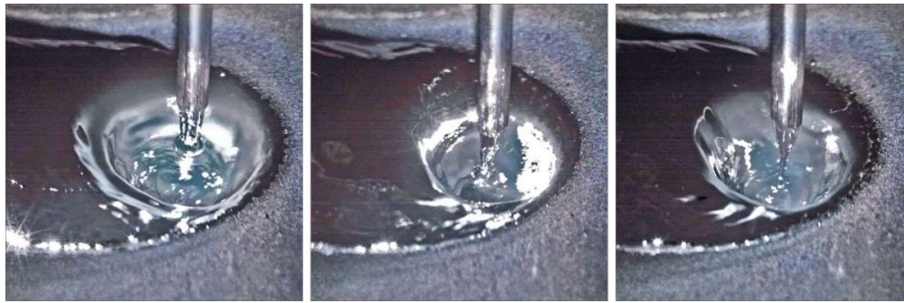
Figure 2 – Crater created by arc pressure on the weld pool. Tests carried out in bead on plate conditions.
