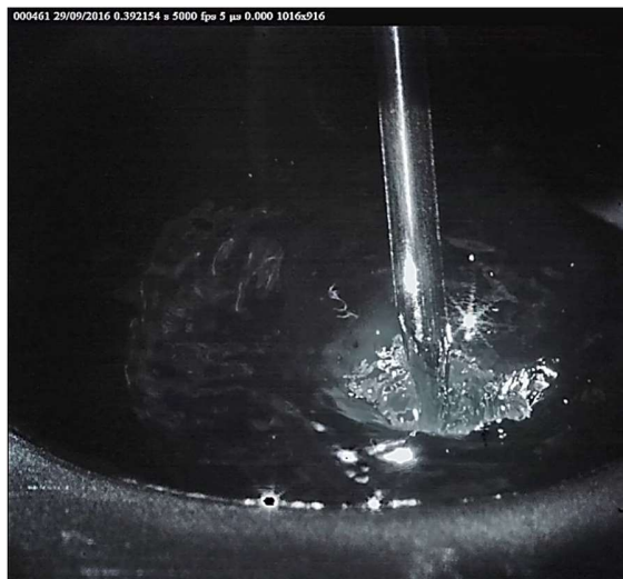
Figure 3 – Crater instability during short-circuiting due to an inadequate inductance adjustment (high speed video on LABSOLDA'S Channel on – https://youtu.be/zCr5Imyf4fM ).
