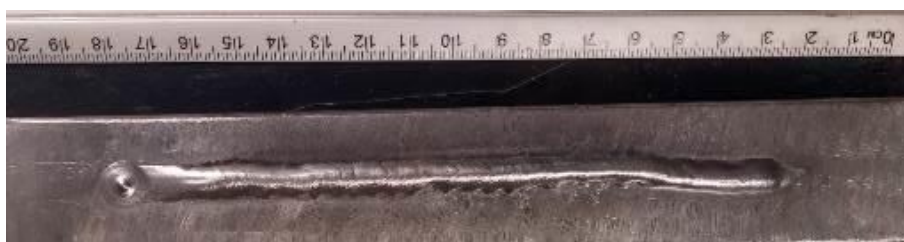
Figura 10 - Teste com HotWire - 150A. V_s = 30\text{cm/min} e V_a = 3,4\text{m/min}
