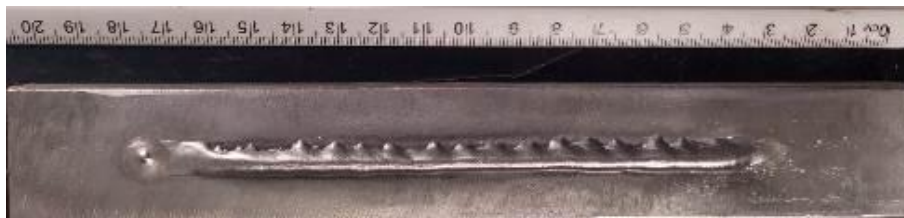
Figura 6 - Teste com ColdWire, V_s = 30\text{cm/min} e V_a = 3,4\text{m/min}
