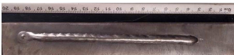
Figura 8- Teste com HotWire - 75A. V_s = 30\text{cm/min} e V_a = 3,4\text{m/min}
