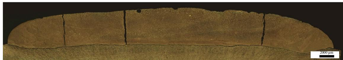
Figure 12: Cross section panorama of hardfacing with DURMAT FD 61 1.6mm over S235 steel. Light microscopy 25x. Etched with Oberhofer. Scale bar = 2000 μm
