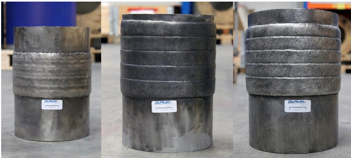
Figure 8: Three 7" pipe sections hardfaced with three different flux-cored wires.: (A) Nickel basis, (B) Iron basis, (C) Cobalt basis. Scale: 30 mm.
