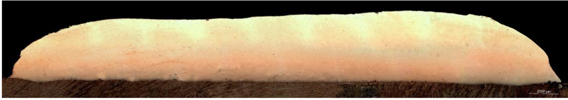
Figure 15: Cross section panorama of hardfacing with DUROLIT 6, 1.6mm, over S235 steel plate. Light microscopy 25x. Etched with Murakami.
