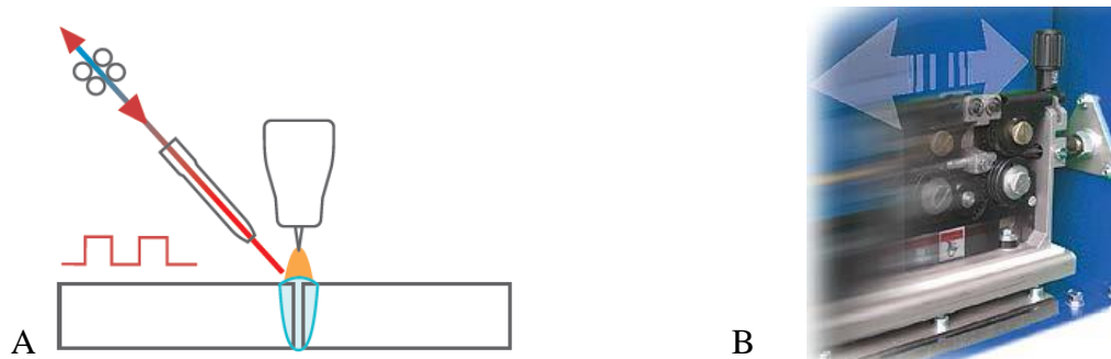
Figure 3. TIG process with dynamic wire feed - A- Schematics of the wire movement (adapted from [11]); B - Oscillatory movement of the traction mechanism [13]
