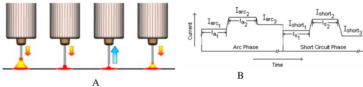
Figure 2. MIG / MAG process with dynamic wire feed; In A - Representation of the movement of the wire [6]; In B - Schematic diagram of the current cycle [9]
