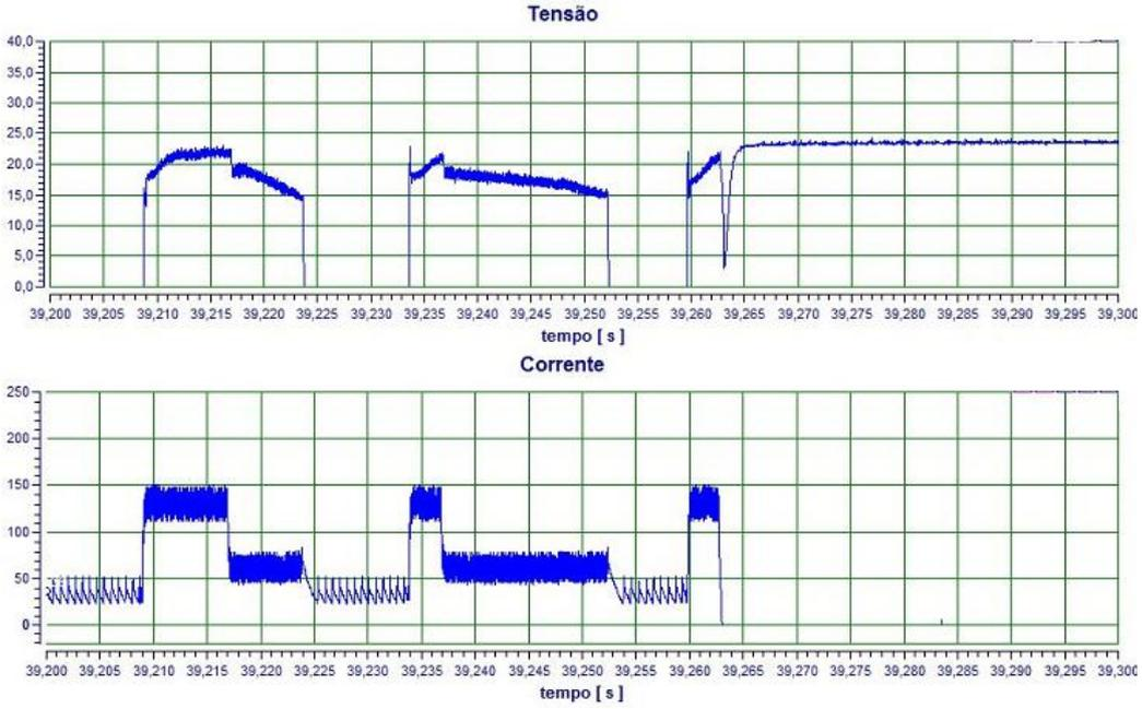
Figure 8 - Voltage and current oscillograms with highlight for the finishing stage
