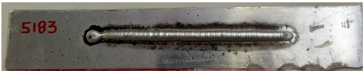
Figure 10 - Bead # 2, ER5183 aluminum wire, 1.2 mm in diameter
