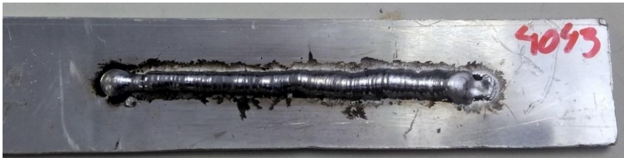
Figure 9 - Bead # 1, ER4043 aluminum wire, 1.2 mm in diameter
