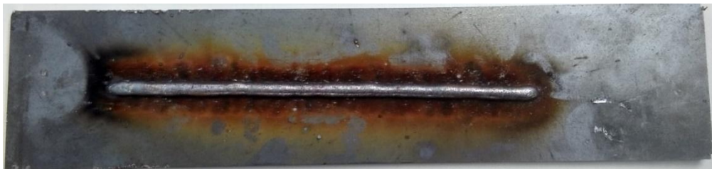
Figure 12 - Bead # 3, steel wire ER70S-6, 1.2 mm diameter
