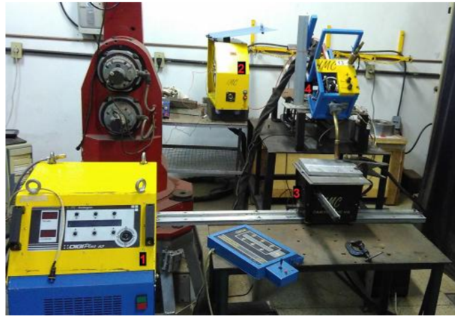
Figure 5. Test rig layout with : welding power source; Manipulator for piece displacement; Prototype torch for dynamic wire feed
