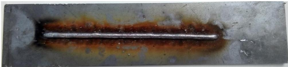
Figure 12 - Bead # 3, steel wire ER70S-6, 1.2 mm diameter
