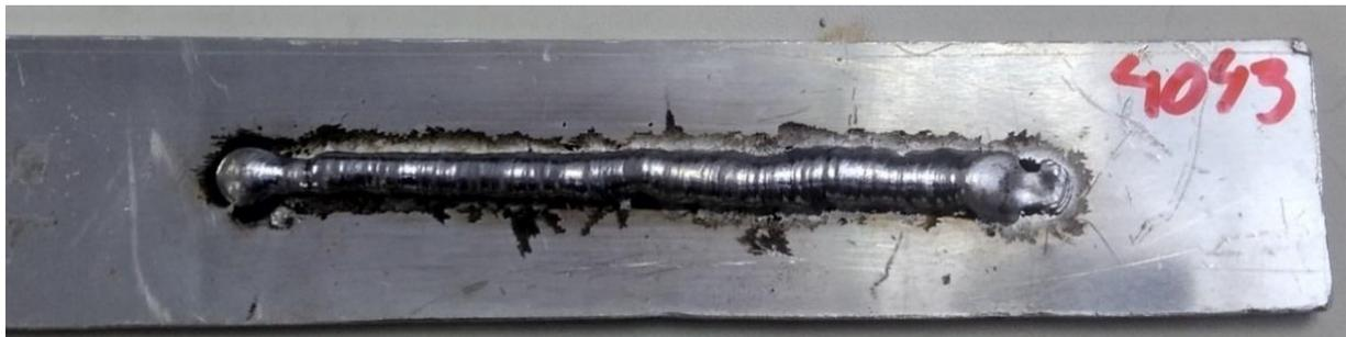
Figure 9 - Bead # 1, ER4043 aluminum wire, 1.2 mm in diameter
