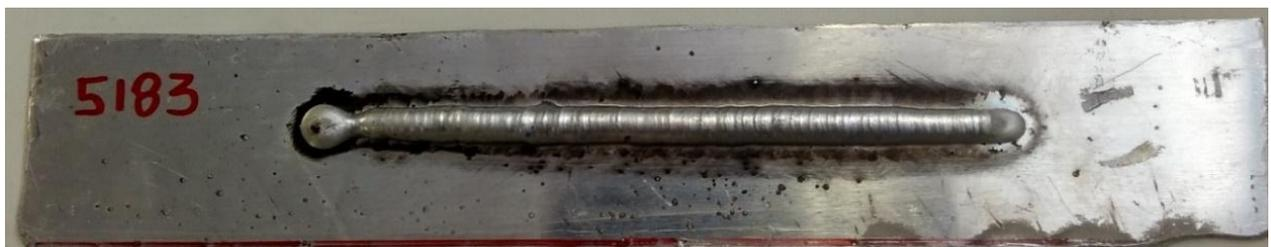
Figure 10 - Bead # 2, ER5183 aluminum wire, 1.2 mm in diameter
