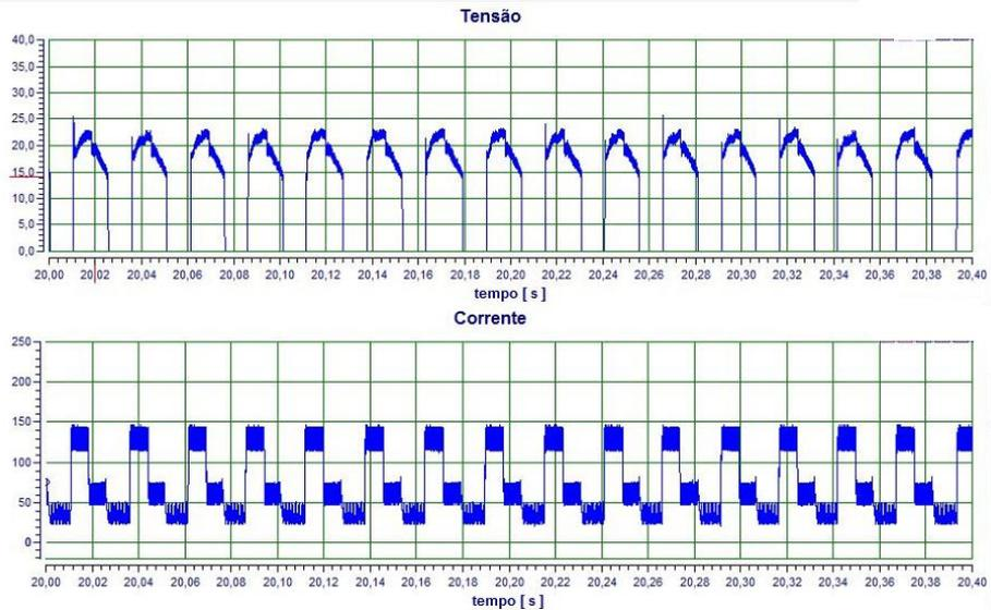
Figure 7 - Voltage and current oscillograms with highlight to the welding steady state stage, in weld made with ER5183 aluminum wire with  $\varnothing = 1,2 \text{ mm}$
